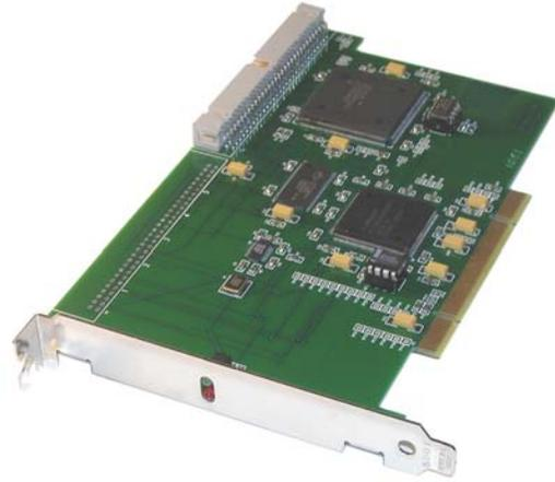
The BQP-2300 works with *Logical's* PCI-based option modules to allow users to migrate from a Qbus system to a PCI-based system while maintaining their investment in software and user equipment. The BQP-2300 can be used with *FutureVAX* for a complete plug-and-play solution.
